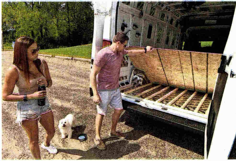
In this summer of 2021 image Erica Battle and Nick Kokenos show off how they're placing particle board under and around their Ram ProMaster conversion van to place insulation in it to keep them cool in the summer and warm in the winter. JOHN HEIDER/HOMETOWNLIFE.COM
