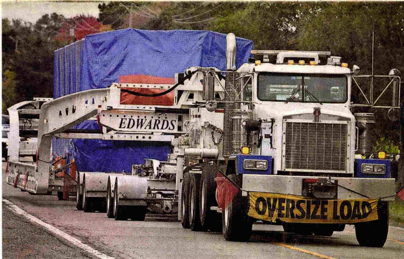
The 200,000-pound compressor is hauled along Haggerty Road in October. COURTESY OF ROAD COMMISSION FOR OAKLAND COUNTY
