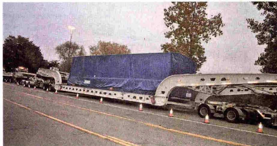
The flatbed trailer carrying the compressors is 170 feet long.
