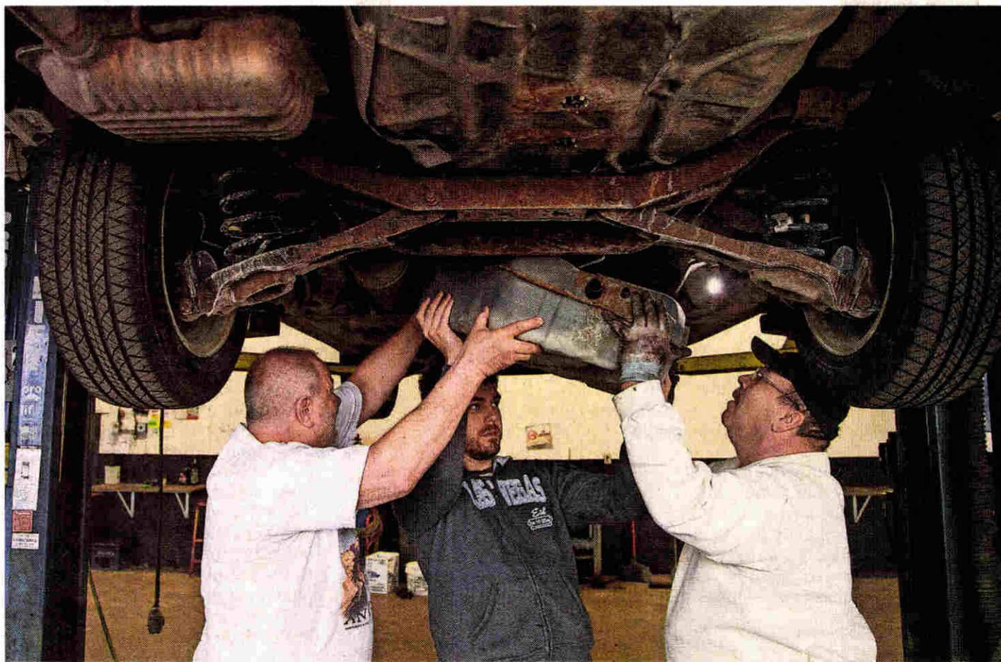
Under a lift, from left, Jerry Carson, his son Andrew, both of Canton, with their friend Dewie Smith of Northville, carefully drop the gas tank off Andrew's 2007 Ford Focus at My Mechanics Place in Livonia, April 11. They have to remove the gas tank from the car in order to replace the fuel pump.
