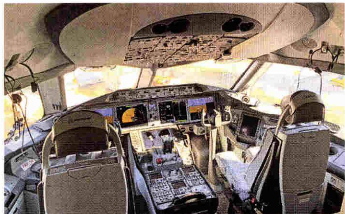
The controls in newer cockpits, such as United's Boeing 787-10 Dreamliner, have more touchscreens to replace switches and buttons. BEN MUTZABAUGH/USA TODAY
