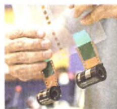
Film is taped to a plastic card that pulls the film through the developing processor.
