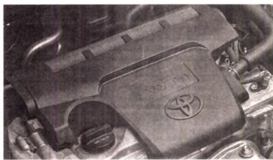
RAV4 is powered by a 2.5-liter, 4-cylinder engine.
