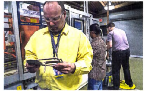
Bryan Palmer examines a finished part for problems. Students Mohammed Mogally and Blake Woolner run the injection molding press.
