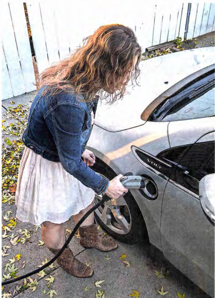
Elissa Potter plugs in Daisy to the 220v home charging station. A full charge takes about four hours at the station.
