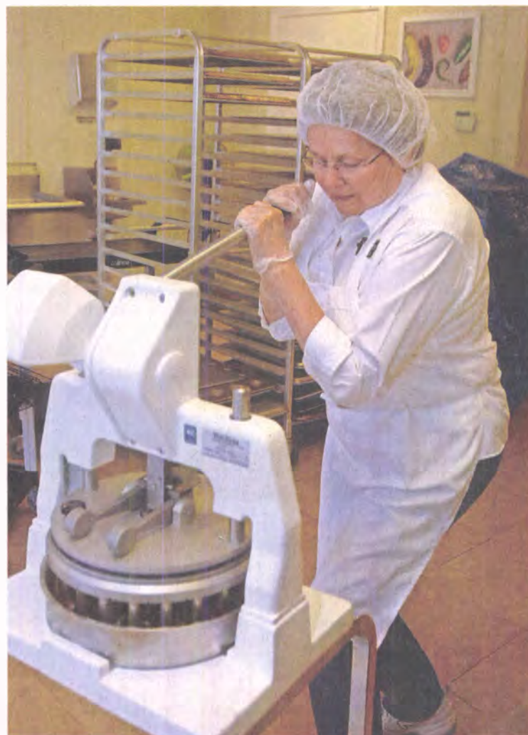
Using a machine sure beats scooping dough by hand. Julie Tenbusch presses the lever on a dough-cutting machine
