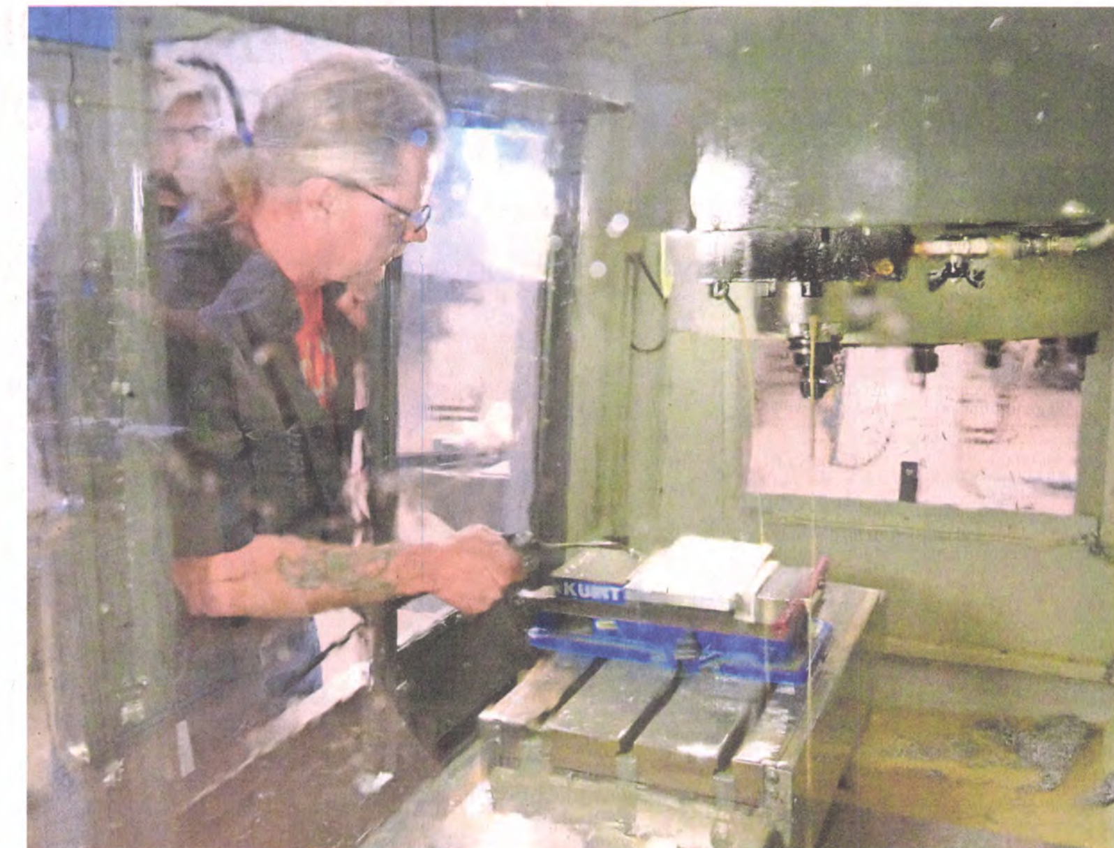
Instructor Mark Schaffroth clears metal chips and coolant from a block of aluminum that is machined by a vertical CNC mill.
