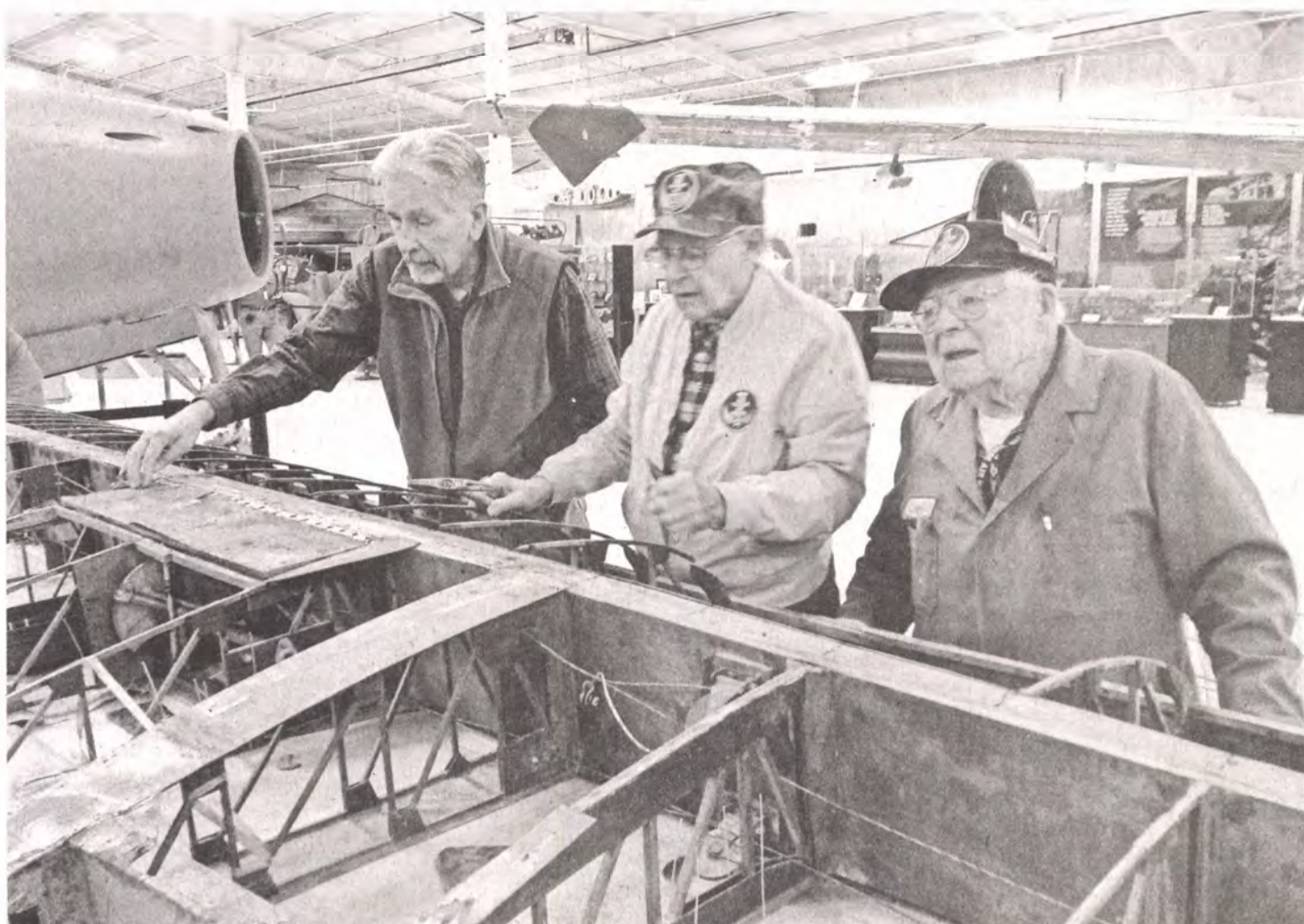
Restoration manager Ralph Koehler of Livonia (from left), Joe Kosek of Westland and Gene Blanchard of West Bloomfield look at how to remove a spoiler from the wing of a TG-3 glider that's being restored at the Yankee Air Museum.
