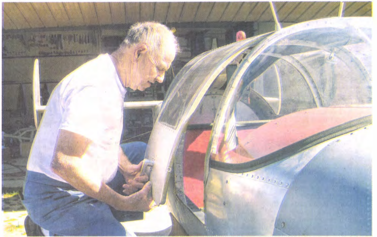
Marvin Dunlap of Green Oak Township opens the door he cut into his prototype 1947 four-seat Ercoupe, which never made it off the factory floor. Dunlap used old blueprints and designs to assemble the plane.
