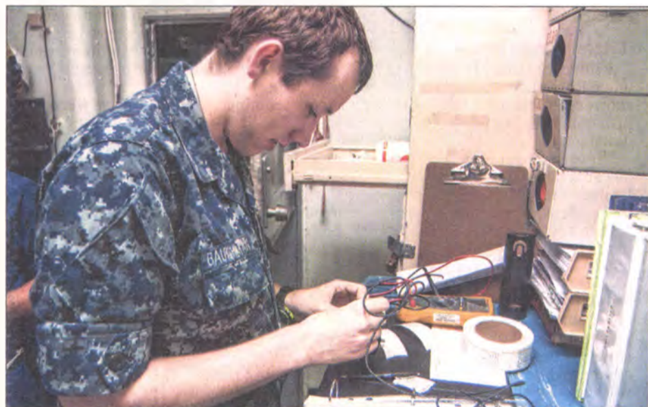
Electrician's Mate 3rd Class Nicholas Baughman of Westland uses a fluke meter to verify the electrical safety of a charger in the electrical safety office aboard the U.S. Navy's forward-deployed aircraft carrier USS George Washington. The carrier and its embarked air wing, Carrier Air Wing (CVW) 5, provide a combat-ready force that protects and defends the collective maritime interest of the U.S. and its allies and partners in the Indo-Asia-Pacific region. U.S. NAVY PHOTO BY MASS COMMUNICATION SPECIALIST SEAMAN APPRENTICE OSCAR ALBERT MORENO JR.
