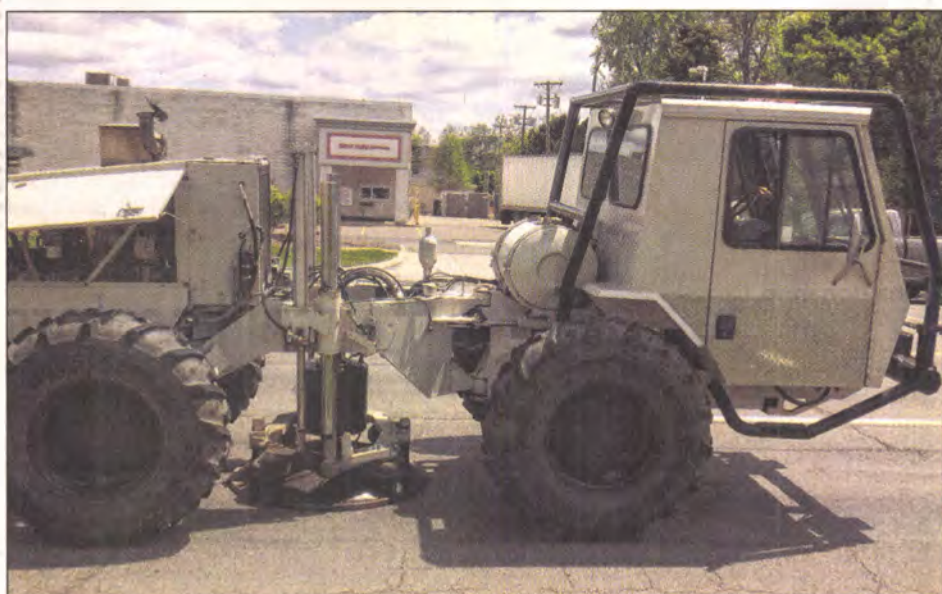
A vibrator truck collects data for a seismic study along Beech Daly Thursday.
