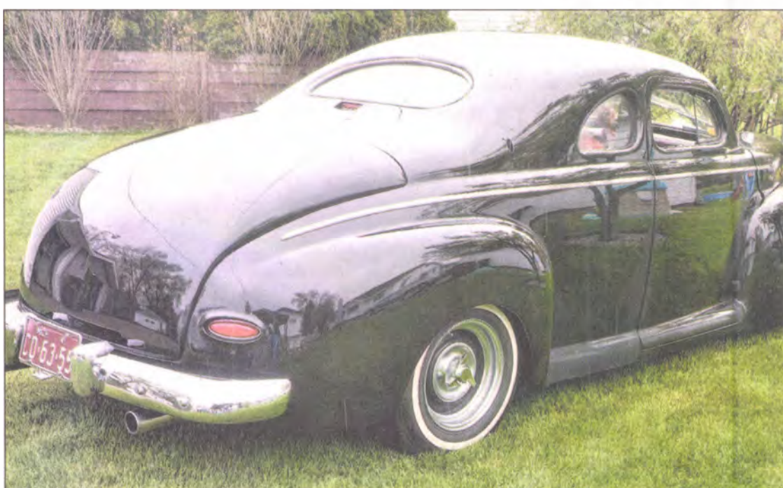
The 1941 Ford business coupe spent years upside down in a swamp in South Dakota. Bob Hayes had the vision and resurrected the car, chopping the top 5½ inches, adding grillwork from a 1950 Oldsmobile, seats from a 1980 Thunderbird and powering it with a 1951 flathead Ford V-8.
