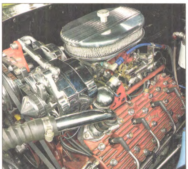
The 1941 Ford business coupe features a flathead Ford V-8 that came out of Bob Hayes' other street rod, a 1951 Ford Victoria.
