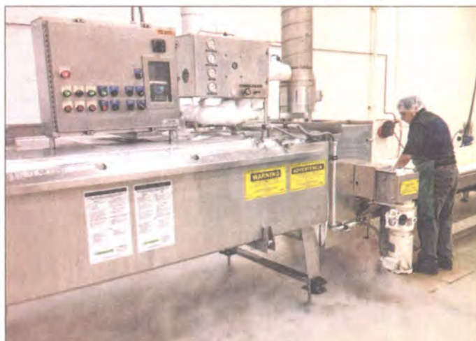
Jorge Hernandez stands at the end of a machine that freezes the ravioli to minus-137°F before it is packed into five-pound boxes.
