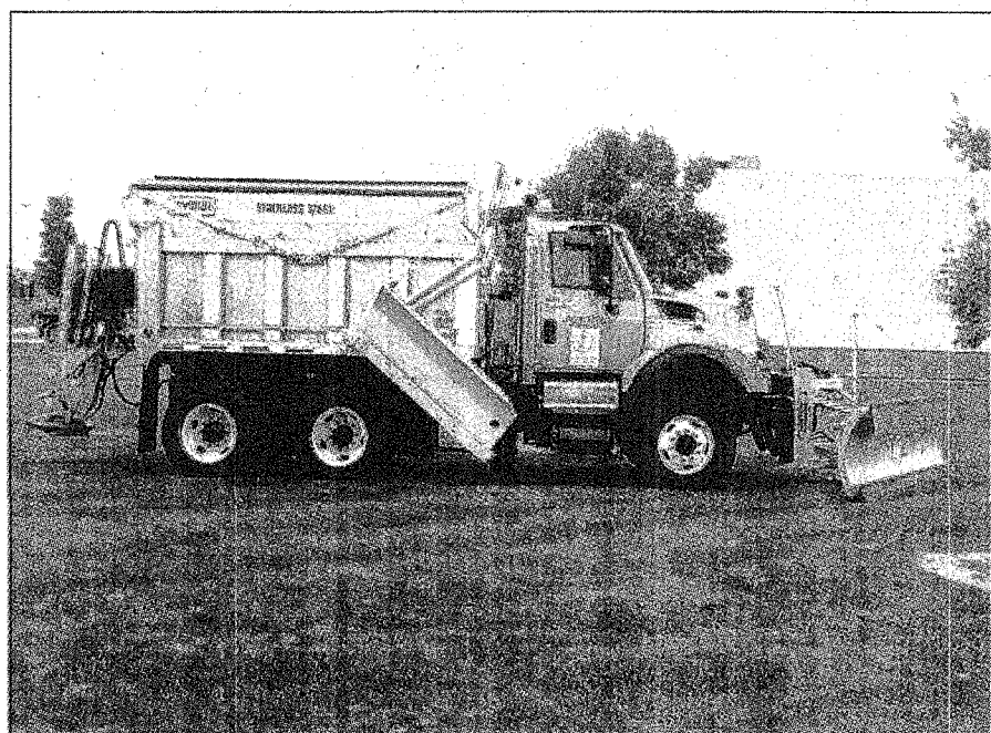
County road officials hope to double the amount of snow they can clear at one time with the new 6-foot wide wing plows installed on the sides of their trucks.
